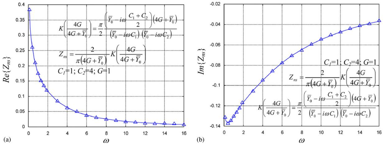
Fig. 9. Real (a) and imaginary (b) part of the node–substrate impedance  $Z_{ns}$  versus the values of  $\omega$ : comparison between theoretical (continuous line) and Monte-Carlo results (triangles). The plots refer to a grid where the conductances of the lattices are all fixed at a given value  $G = 1$  and the capacitors towards the substrate are randomly placed. Each capacitor is placed into the network assuming the value 1 with probability 1/2 and the value 4 with probability 1/2.
