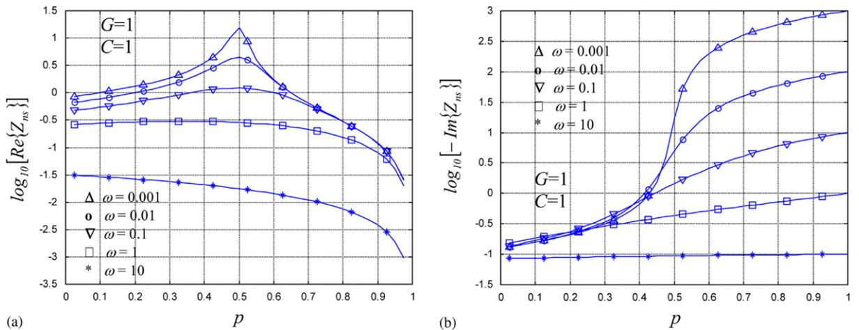
Fig. 11. Real (a) and imaginary (b) parts of the node substrate impedance  $Z_{ns}$  (in logarithmic scale) for the frequency controlled percolative network. The graphs are shown in terms of the probability  $p$  for different values of the frequency. A comparison between theoretical (continuous line) and Monte-Carlo results (symbols) has been drawn.
