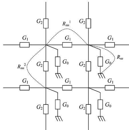
Fig. 1. 2D version of the general topology network used in this work. One can observe the anisotropy of the network and the definition of the characteristic node–node and node–substrate resistance.
