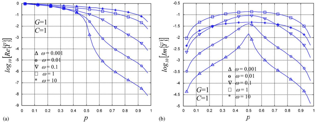
Fig. 10. Real (a) and imaginary (b) parts of the equivalent admittance  $\bar{Y}$  (in logarithmic scale) for the frequency controlled percolative network. The graphs are shown in terms of the probability  $p$  for different values of the frequency. A comparison between theoretical (continuous line) and Monte-Carlo results (symbols) has been drawn. In the case of extremely low frequency the breakdown of the real part appearing for  $p = 1/2$  represents the percolation phenomenon.
