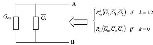
Fig. 5. Scheme that defines the relation between the Thevenin conductance  $G_{eq}$  introduced in Fig. 4 and the characteristic resistance values  $R_{m}^k = R_{m}^k(\bar{G}_0, \bar{G}_1, \bar{G}_2) \forall k$  and  $R_{ns} = R_{ns}(\bar{G}_0, \bar{G}_1, \bar{G}_2)$ .
