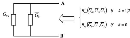
Fig. 5. Scheme that defines the relation between the Thevenin conductance  $G_{eq}$  introduced in Fig. 4 and the characteristic resistance values  $R_{m}^k = R_{m}^k(\bar{G}_0, \bar{G}_1, \bar{G}_2) \forall k$  and  $R_{ns} = R_{ns}(\bar{G}_0, \bar{G}_1, \bar{G}_2)$ .
