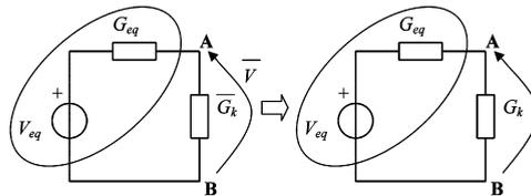
Fig. 4. Thevenin equivalent circuit between two adjacent arbitrary nodes of the lattice before and after the substitution of the effective conductance  $\bar{G}_k$  with a particular random instance  $G_k$ .
