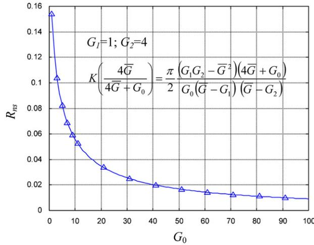
Fig. 6. Theoretical (continuous line) and Monte-Carlo results (triangles) for a grid where the conductances of the lattices are randomly placed and the conductances of the substrate are all fixed at a given value  $G_0$ . Each conductance of the grid is placed into the network assuming the value 1 with probability 1/2 and the value 4 with probability 1/2. The node–substrate resistance  $R_{ns}$  of the network is represented versus the values of  $G_0$ .
