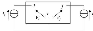
Fig. 2. Scheme of the lattice network where two arbitrary nodes and the substrate node are considered and connected to the current generators described in the main text.
