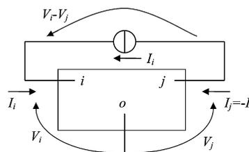
Fig. 3. Particular configuration of the network introduced to define the node–node resistance. Here the substrate node is an unconnected terminal.
