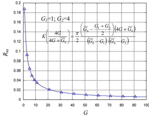
Fig. 7. Theoretical (continuous line) and Monte-Carlo results (triangles) for a grid where the conductances  $G$  of the lattices are fixed and the conductances of the substrate are randomly assigned. Each conductance toward the substrate is placed into the network assuming the value 1 with probability 1/2 and the value 4 with probability 1/2. All the grid conductances are fixed to the value  $G$ . The node–substrate resistance  $R_{ns}$  of the network is represented versus the values of  $G$ .
