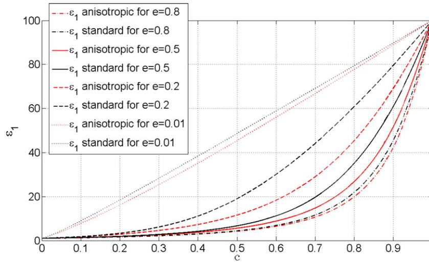
**Figure 4.** Comparison among the results for  $\epsilon_1$  obtained with the anisotropic differential system (62) and the standard differential method (63). The solutions of equations (62) are placed under the corresponding solutions (63).
