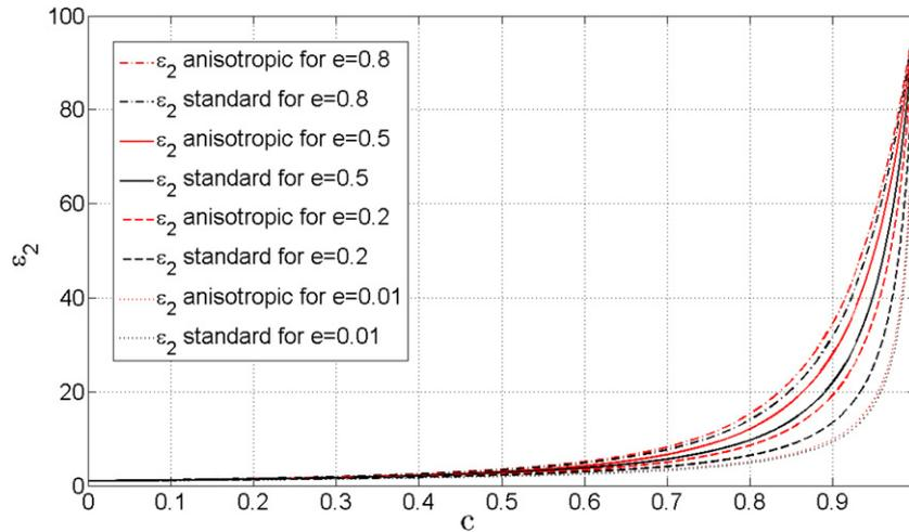
**Figure 5.** Comparison among the results for  $\epsilon_2$  obtained with the anisotropic differential system (62) and the standard differential method (63). The solutions of equations (62) are placed above the corresponding solutions of (63).
