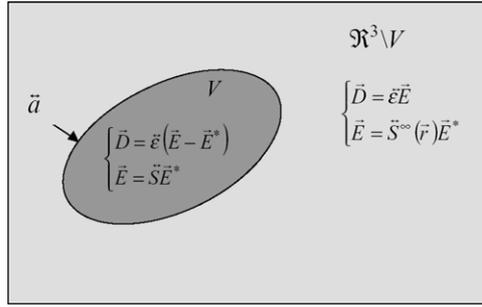
**Figure 1.** Scheme of an inclusion  $V$  with eigenfield  $\vec{E}^*$  embedded in an anisotropic environment. The results in terms of the interior points and exterior point Eshelby tensors are also shown.
