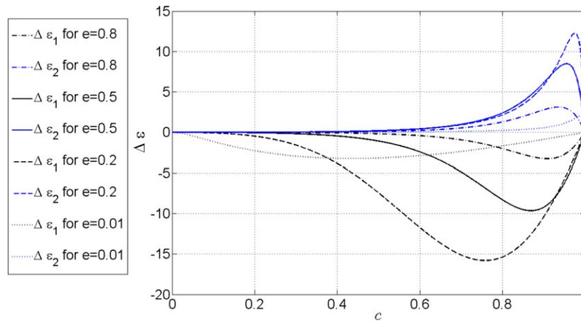
**Figure 6.** The variations  $\Delta\epsilon$  (values obtained with equation (62) minus values obtained with equation (63)) are plotted versus the volume fraction  $c$  of the composite material. One can see that the relative error can assume values up to 20%.
