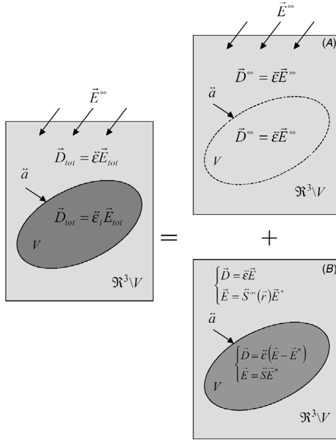
**Figure 2.** Scheme of the equivalence principle between the inhomogeneity problem and problem A (homogeneous medium) superimposed to problem B (inclusion as reported in figure 1).
