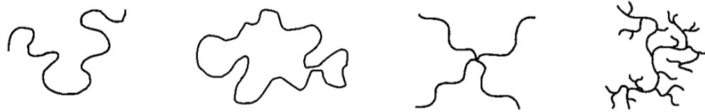
Figure 1.1: **Different types of polymer architectures.** Linear, ring, star-branched and randomly-branched polymers. Taken from: Ref. [16]
