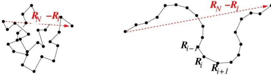
Figure 1.22 – Diagram of comparison between FJC (on the left panel) and WLC model (on the right panel).
