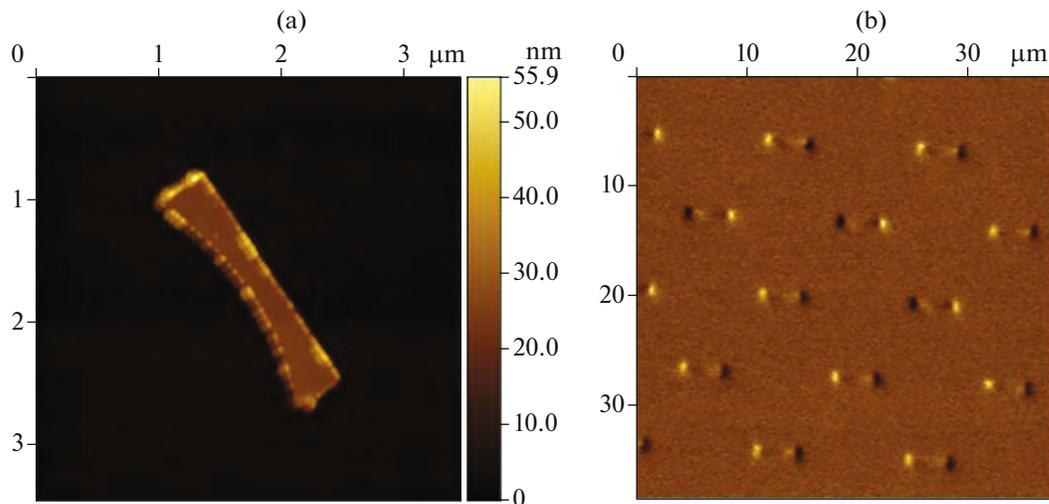
**Fig. 2.** (a) Topography of a magnetoelastic nanostrip with a parabolic profile (atomic force microscopy) and (b) an array of such nanostrips on a piezosubstrate (magnetic force microscopy).
