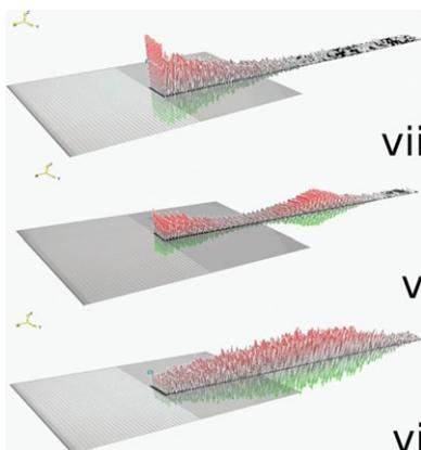
Surface phonon cavity formed by the placement of a defect of a single domain within periodic domain inversion of single crystal piezoelectric lithium niobate exhibiting surface phononic bandgap through the phonon-polariton coupling is introduced. It is shown that the proposed cavity can exhibit entrapment of phonon-polariton, indicated by the simultaneous localization of both surface phonons and the electric within the defect.
