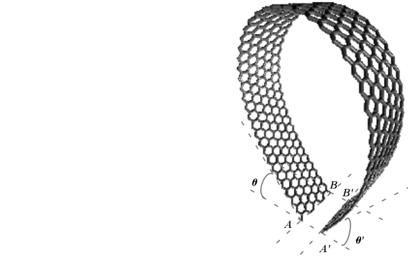
Figure 8.4: For instance we show a relaxed atomic configuration for a nanoribbon of graphene bended with parallel fixed edges and attach angles free. The edges \overline{AA'} and \overline{BB'} are kept parallel and at fixed distance a , while the attach angle \theta are free.
